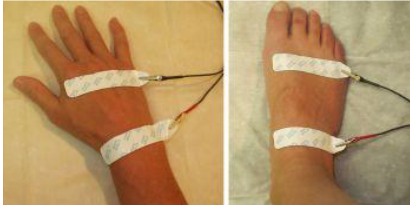
Fig. 4 Adhesive electrodes for XITRON 4200 on hand and foot
